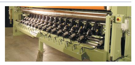
**MOTOR DRIVEN** bottom knife systems are capable of automatic and immediate changing of slit widths without stopping the slitting action. This capability has been successfully employed to retain slit width accuracy when responding to tracking camera signals on high speed packaging print lines.
