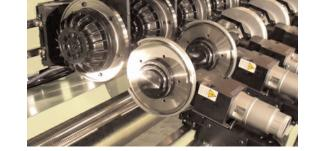
**SHAFT DRIVEN** QUICK SET systems bottom knives mount to precision traversing carriages that prevent excessive axial run-out and shaft deflection. This capability allows for unlimited shaft lengths,
