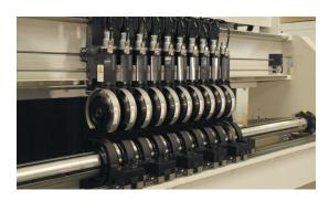
**DIENES EASY TRIM** shear slitting systems, employing QUICK SET technology, are designed specifically for effortless and trouble-free change of trimmed web widths.
